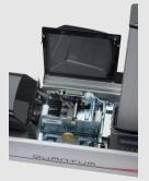
Reversible upper and lower encoding units for magnetic stripes and contact smart cards
